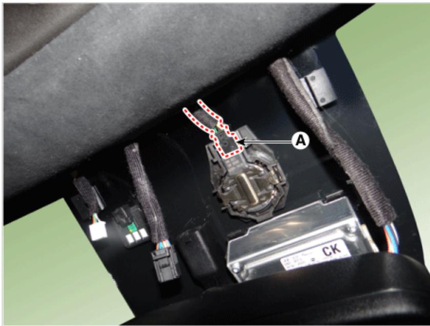
3. Be careful not to damage the cover latch by applying excessive force. To remove the bracket, pull the holes of the bracket outside using a small flat-head screwdriver (A).
