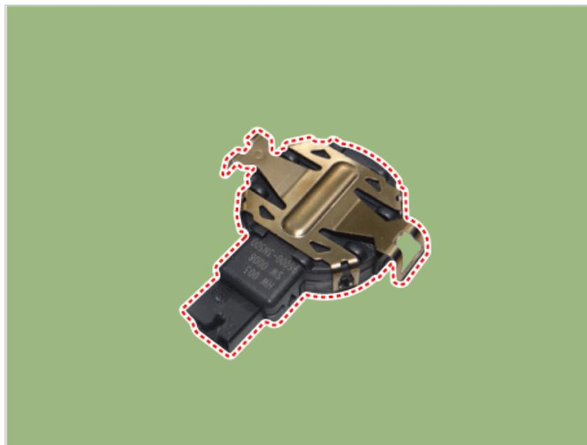
4. Rain sensor module is attached to the front windshield by glue. When replacing the front windshield, remove the rain sensor module from the existing front windshield and install it on the new front windshield.
